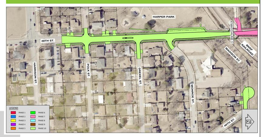
KEEP OMAHA **moving**  Phase 10 is the final phase of construction and shown here in light green. This phase includes construction of 48th Street south of the BNSF railroad tracks and the cul-de-sac on Madison Street.
