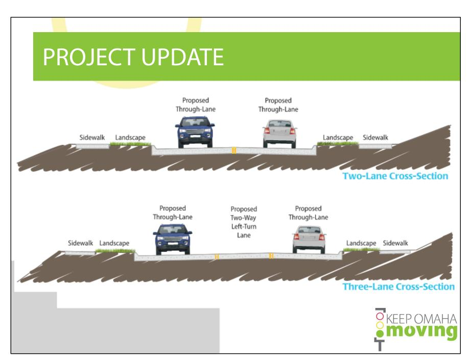
This graphic shows the typical cross section of the proposed 2-lane and 3-lanes sections on 48th Street and Q Street. The 3-lane section consists of one through lane in each direction and a center left-turn lane.
