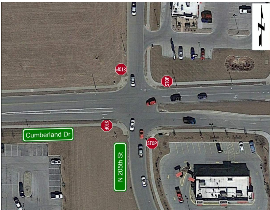
Figure 10. All-Way Stop Control Alternative (Near Term Only)
