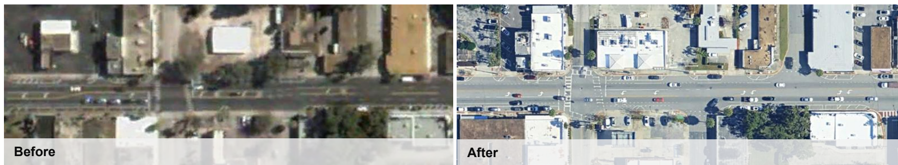
Figure 7: Edgewater Drive Before and After Lane Reconfiguration
