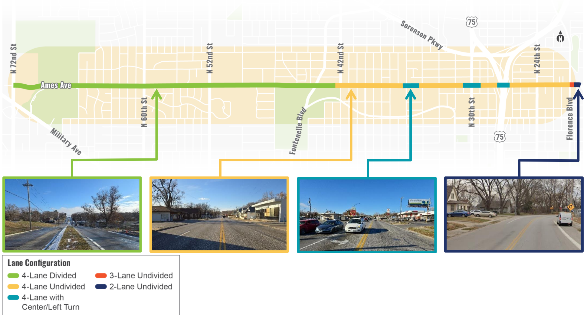
Figure 2: Existing Typical Lane Configurations
