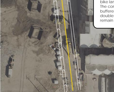
bike lanes for approximately 2 miles. The concept proposes striping wide buffered bike lanes. The existing double yellow centerline striping will remain in place.
